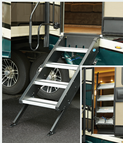
Sturdy and lightweight entry steps stay clean and free of travel damage because they are housed inside the unit during transport.
