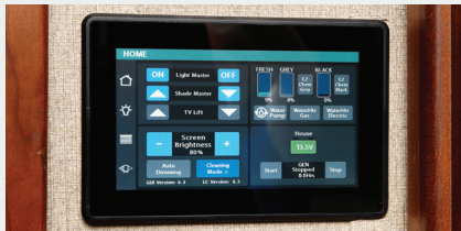
Firefly Integrations touch screen panel provides controls for lighting, tank monitoring, awnings, slides, and heating and air-conditioning.
